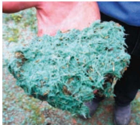
FIGURE 3.7: An example of what hydromulch looks like close up (Photo Lester Piggott).
